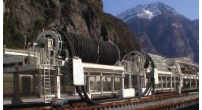
Giant tunnelling reels for the San Gothard tunnel, Switzerland
